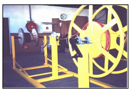
The all-in-one hand turned coiling machine was first designed for the medium sized electrical wholesaler. This machine is ideal for decoiling small lengths from a 300 meter drum and will also accept drums used in the cellular communications industry. This machine is capable to coil any form of flexible tubing, rope, hose etc.
